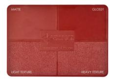
As one piece, this plastic plaque is the same color but with a different color appearance dependent on the degree of surface roughness in each quadrant.
